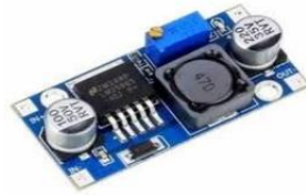
Gambar 2.4. Modul Step Down LM2596 [19]
