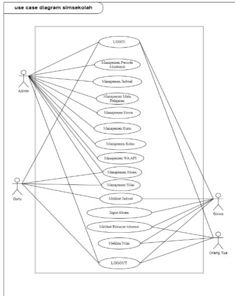
Gambar 2. Use Case Diagram
